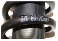
Example of our spring rate notation: 220-60 (70mm) in which: 220 = length in mm 60 = N/mm or Kg/cm (70mm) = Inner diameter in mm (if this diameter is not listed on the spring it is the standard diameter of 60mm)
